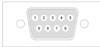
Figure 11: DB9 connector, for optional -RC# remote communications
