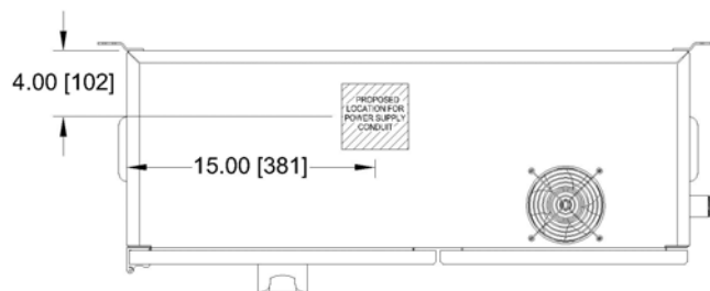
Figure 8: Recommended location for power supply conduit (72kW unit shown)
